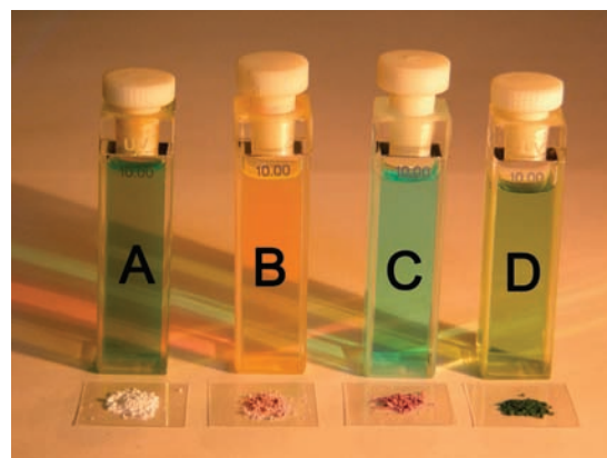
Figure 3. \text{TiO}_2 powders labeled with dyes 2 , 10 , and 7 and their dichloromethane solution. Solution A is an equimolar solution of the phenyliodo BODIPYs 11 , 12 , and 13 . Solutions B , C , and D are micromolar solutions of the acacH dyes 2 , 10 , and 7 . The bottom glass slides contain the dry powders of \text{TiO}_2 which have been treated from left to right with solutions A , B , C , and D , respectively, highlighting the covalent linking of the dye to the semiconductor.
